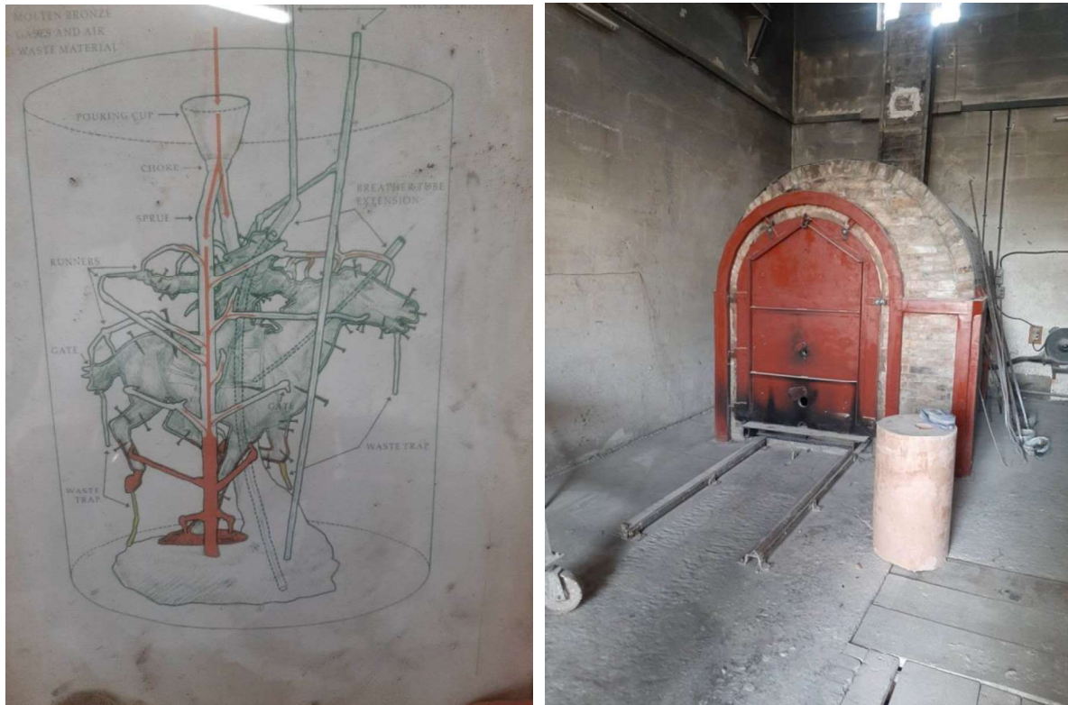
Figure 3 - Wax rods and plaster encasement and the kiln
