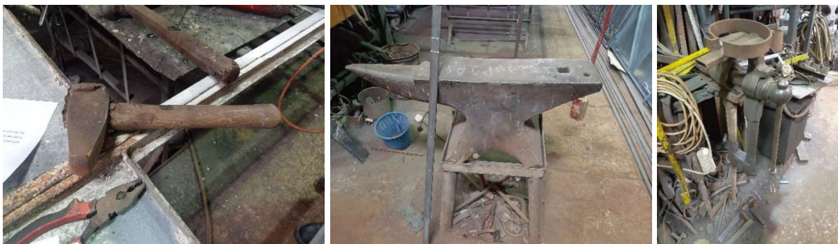
Fig 10 - The hammer, the anvil and the leg-vice
