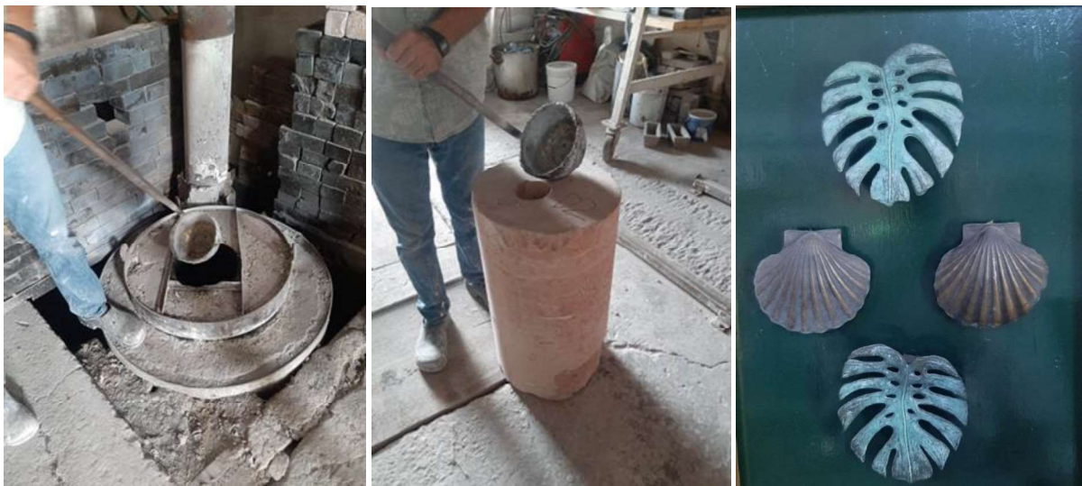
Figure 4 -Pouring melted bronze. Figure 5 - Different finishes
