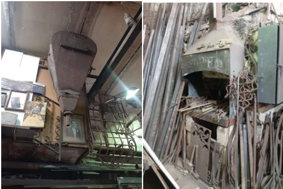
Fig 11 - The hand blower and the coal forge
